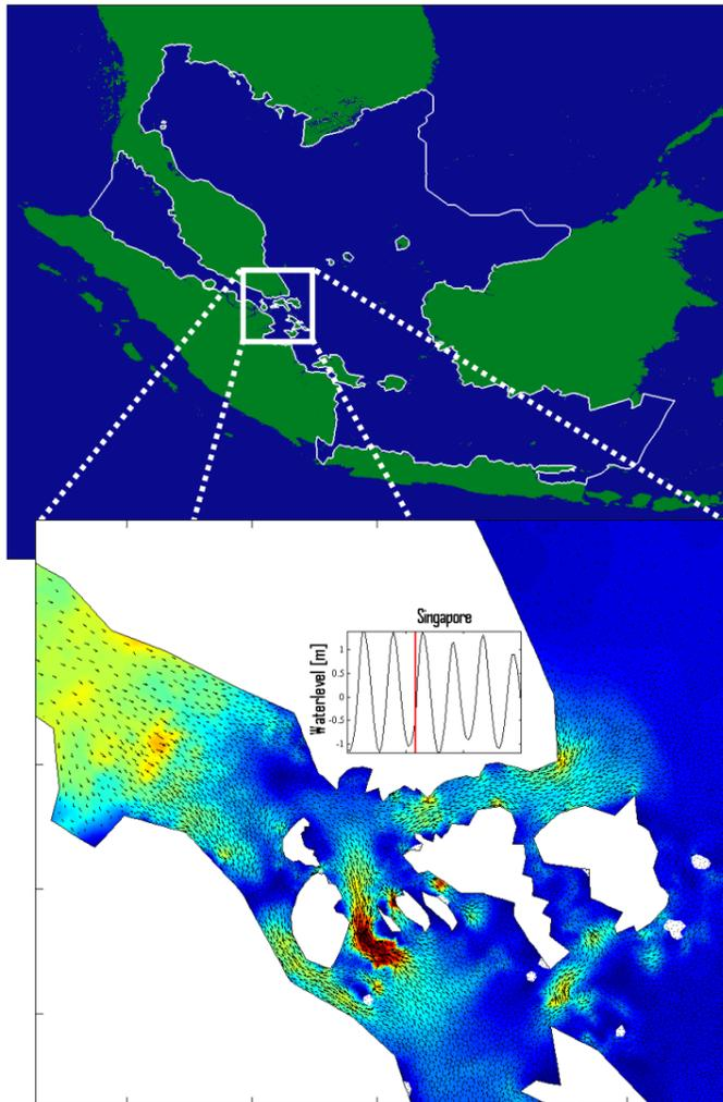
The boundaries of the South East Asia Model are indicated by the thin white lines in the upper figure. The inset shows flow velocities around Singapore during flood current.
