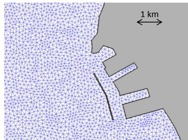
Whenever the region of interest is located within the boundaries, the model can be adjusted to fit the required grid resolution. Here a refinement is shown for Laem Chabang, the biggest port of Thailand.
