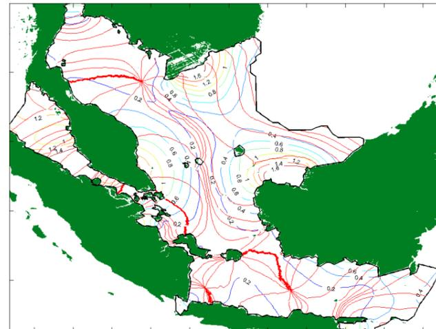
Amphidromic system in South East Asia, consisting of lines indicating equal tidal phase and equal tidal range.
